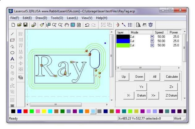
Use the "Offset Curve" menu command or the toolbar button to offset the new guide shape three times. The offset distance should be about 1mm.
