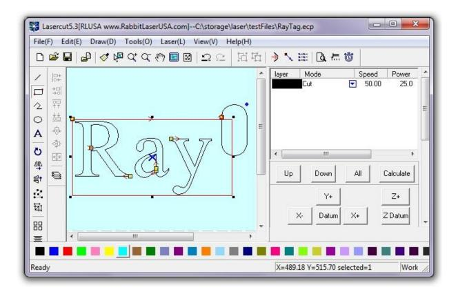
Draw a rectangle around the name. This rectangle will be used as part of a guide for the rest of the project. Make sure the rectangle does not cut off part of the name or leave too much awkward space.
