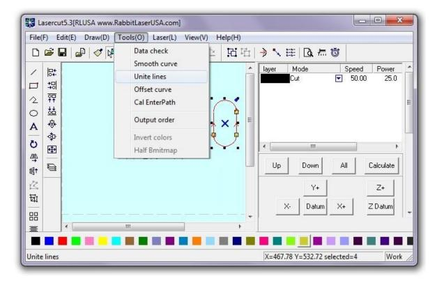
Select all the line segments for the slot. Use the "Unite Lines" command to make these segments into one polyline.
