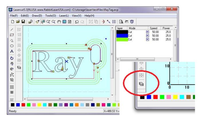
The guide object is no longer needed. We can delete this object or make it a new color such that the new color layer can be turned off, locked, frozen, or hidden. I normally choose to hide the guide object in a different color layer. The "Layer Control" button is located at the bottom of the left toolbar.
