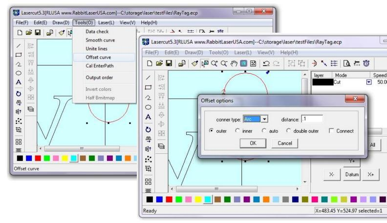
Select the slot shape. Use the "Offset Curve" menu command or the toolbar button to create another slot. Use an offset distance of only 0.1 mm for the new offset distance. The shape that we will create will be an arc on the outside of the existing shape. The new slot will be used as a guide for other parts of the project.
