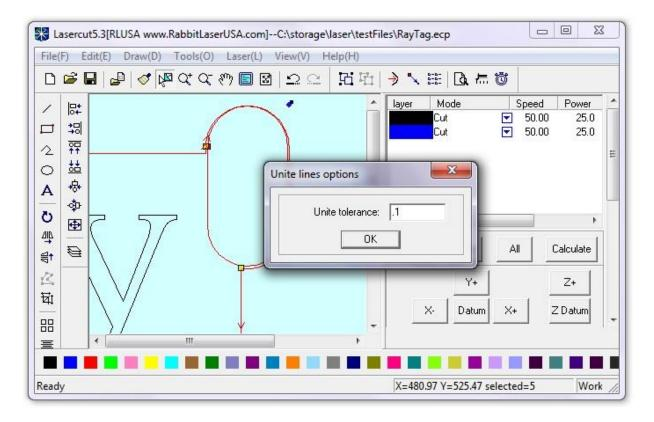
Remember how we used the "Split Line" command. Split the outer slot and the rectangle guide. Use the "Unite Lines" command to make the rectangle and slot into one polygon. This new polygon is our best guide for finishing the tag boundary.
