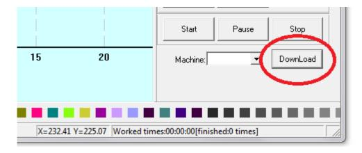
The project is drawn. The laser settings are made. The design project has been saved to file. The next step is "Download" the design into the laser machine. Make sure that the computer is connected to the laser machine by USB cable and that the laser machine is turned on. The computer should already have the drivers loaded.
