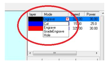
Click on the triangle inside the "Mode" parameter of the black layer. This will expand a small menu of modes that can be used for this layer. You are not required to use any specific color for cutting, engraving...etc. Each project can designate what mode is used on that color layer. For this project, make sure the black layer is used as ENGRAVE by clicking on the "Engrave" option.
