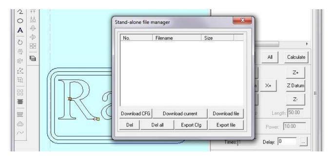
The "Download" command will start a new connection with the laser machine through the "Stand-alone file manager". It is a good practice to delete all files in the laser machine and to download only the current design project. Click on the "Del all" button to erase the laser machine memory. Click the "Download current" to load the circtest.ecp from the LaserCut 5.3 software into the laser machine. The compiled file should be read as xx.mol file extension.
