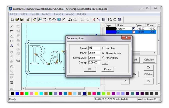
Since the BLUE color layer is set to the "Cut" function, we need to choose some values for the speed, power, and corner power. These values will be determined by your laser machine capabilities and the material properties. The picture shows good starting values for the project. Speed:15, Power:25, and Corner Power:25. The overlap would be used with materials that might have a cut lag while cutting or you are trying to eliminate a laser mark from the start-end cut operation.
