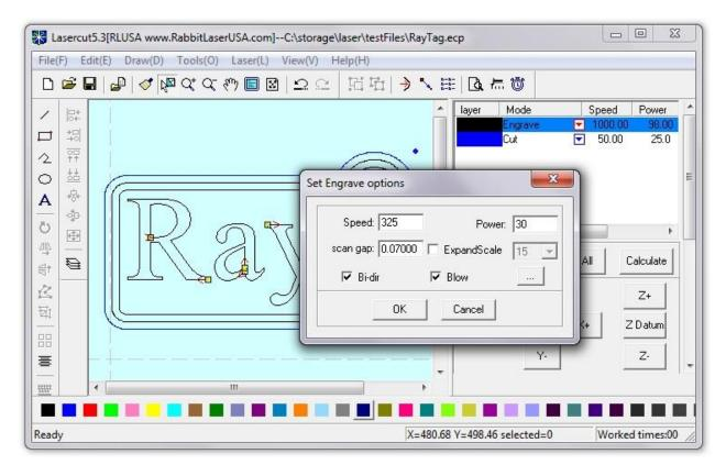
Since the BLACK color layer is set to the "Engrave" function, we need to choose some values for the speed, power, and scan gap. These values will be determined by your laser machine capabilities and the material properties. The picture shows good starting values for the project. Speed:325, Power:30, and ScapGap:0.070
