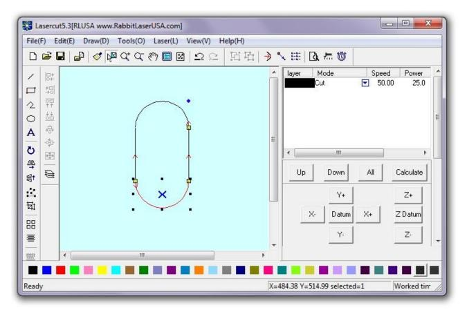
Use the "Draw - Split Line" tool to break the circles apart. Separate the circles at the left and right edges. Once the circles are broken apart, delete the line segments that we do not need.
