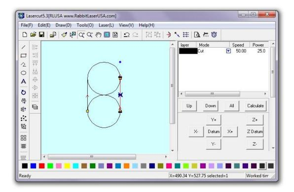
Select the "Draw-Line" tool. Use the snap points to help select the circle start point nodes. Then create the second line by selecting the right set of node points.
