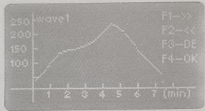
② Following we provide eight different waves, please choose one according to your request. Press the F1/F2 to choose different wave, press F3 to look into different wave parameter, press 4 to confirm the wave you chose.
