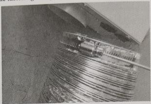
2 Put the exhaust pipe on the product interface, tighten the fastening screws with a screwdriver, and place the exhaust pipe outdoors.
